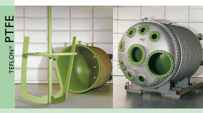
In the spraying sinter procedure (airless and compressed air process), Gutbrod works with Teflon<sup>®</sup> PTFE and Teflon<sup>®</sup> FEP. The coating is sprayed on and then "sintered" at 220° C to 420° C.
